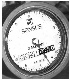
This reads 0021470. If any numbers are in the process of changing, as in this photo where the six is changing to a seven, report the higher number.
